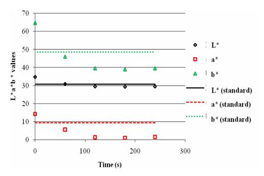
Fig. 4. L\*a\*b values with time and standard L\*a\*b values at 7188 W/m<sup>2</sup> FIR radiation intensity.
